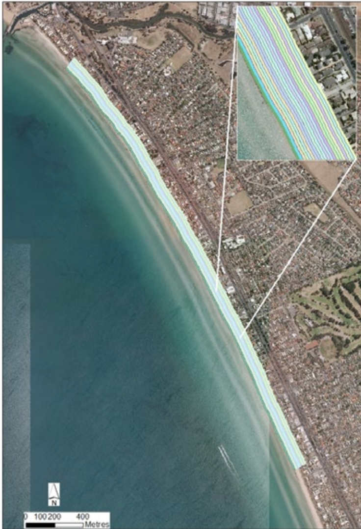
Figure 20: 5m horizontal zones landward of 0m contour AHD to determine width and volume per zone. Insert showing zoomed-in section of the area of interest.
