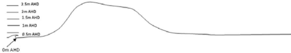
Figure 14: Approach 3 - area and available volume calculations in 0.5m vertical intervals landward from the 0m contour AHD.
